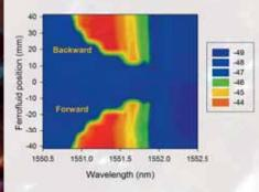
Figure 1. Spectral response of a chirped Bragg grating inscribed in a PCF that is infiltrated using ferrofluid
